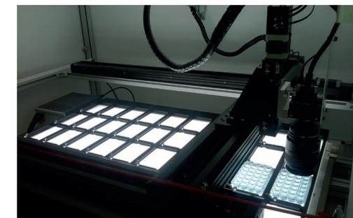
Fig 2. Video acquisition device
